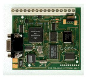
Bitstream Bluetooth-Server BS12 is a complete server equipped with a industrial Bluetooth-modem for wireless connection. The server has a software download feature of code and or parameters within standard software package. Using a standard PC with serial interface, there is no need for separate FLASH programming device.
